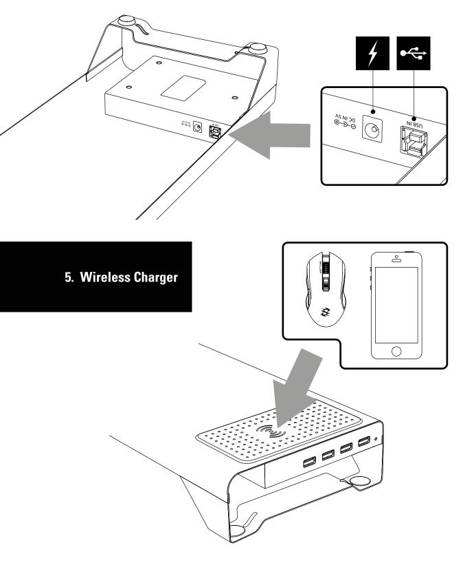
For wireless charging of compatible devices, such as mice or smartphones, place the device centered on the wireless charger. The charging process should start automatically. If not, make sure that there are no resistors, such as smartphone cases, between the charger and the device.
