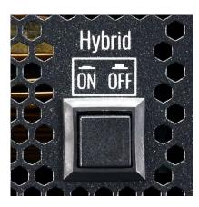
The semi-fanless mode can be manually turned off with the built in analog hybrid switch.
