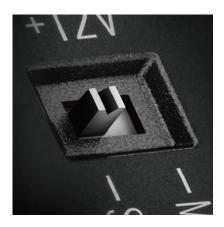
The hardware based rail switch allows you to alter the PSU from single to multiple rails in order to tailor the unit's performance to your needs.
