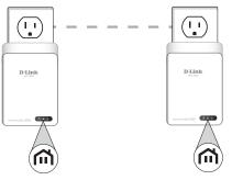
4. To secure your network, press the Simple Connect button for two seconds on one of the adapters. The Power LED will start to blink. Then, within two minutes, press the Simple Connect button on the other adapter for two seconds. Once the Power LEDs stop blinking, verify that the PowerLine LEDs on both adapters are lit (as in Step 3). This indicates that your adapters are properly connected to each other.
