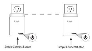
5. You may now connect another device to the DHP-700AV adapter using an Ethernet cable. Verify that the Ethernet LED is lit. Your hardware installation is complete.
