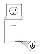
3. Verify that the PowerLine LEDs on both adapters are lit. If they are, the adapters are connected. If not, try another wall outlet (closer to the other PowerLine adapter).
