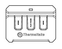
SPEED: Switch over between 2 fan speed modes LED Indicator shows Blue: Normal mode 800~1500rpm LED Indicator shows Red: Low noise mode 400~1000rpm
