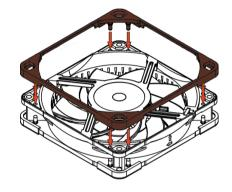
The NA-AVG1 gasket can also be used for other applications that benefit from a tighter seal with the fan.
