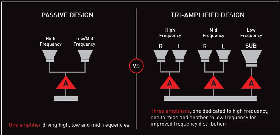
Unlike most conventional soundbars that utilize a single amplifier to reproduce the entire audio spectrum, Sound BlasterX Katana employs three high-performance amplifiers – one dedicated to driving lows, one for mids, and another solely for high frequencies.
