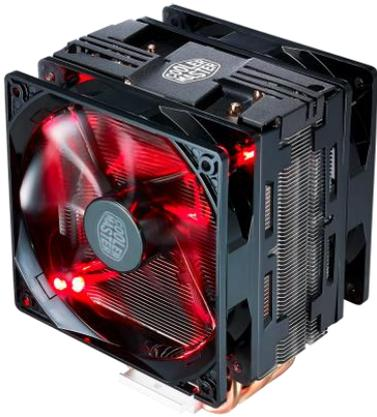
Hyper 212 LED Turbo (Black Top Cover) is equipped with black top cover and dual PWM fans with red LEDs, providing the best balance between airflow and static pressure to take the heat away. Four Direct Contact heat pipes with funnel shaped aluminum fins optimize cooling for optimal CPU performance. Moreover, the improved universal bracket design ensures easy and worry free installation on all platforms.
