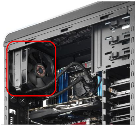
Supports a 120mm radiator in the rear
